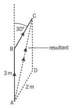
drawing of a scale diagram allows us to measure these. Notice that if the vectors are combined by drawing them in the opposite order,  $\overrightarrow{AD}$  and  $\overrightarrow{DC}$ , these are the other two sides of parallelogram and give the same resultant.
