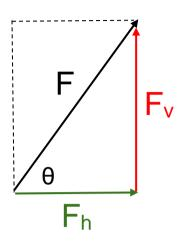
As shown in the diagram, F is the resultant force of  $F_h$  and Fv. If these two forces act together on an object, one pulling to the right ( $F_h$ ) and one pulling upward ( $F_v$ ), then the resultant force, F is pulling up and to the right.
