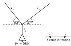
A string or cable can be in tension, but not in compression. If it is in tension, the force pulls on the objects it is attached to. The tension is the same at every point in the cable, or the cable would break, so it is always the same at both ends.
